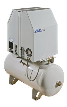
Specifically designed for reliability, energy efficiency, and ease-of-use, there are thousands of Topaz PSA Oxygen Generators currently in use throughout the world. Generating up to 18 LPM (38 SCFH) in a compact package, at up to 95.5% oxygen concentration, the Dual Topaz Plus is a great fit for a wide range of commercial applications.
