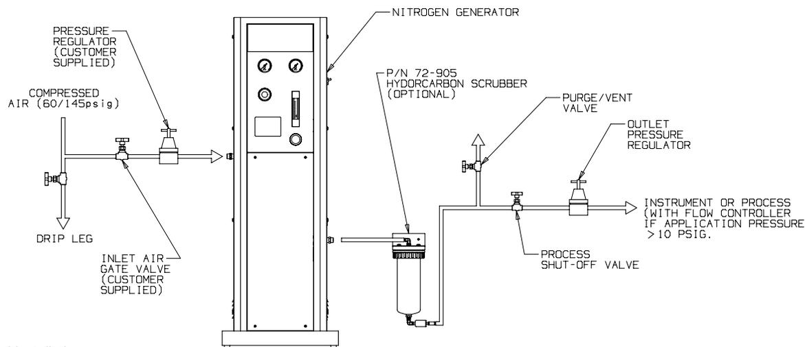
Figure 4 - Recommended Installation
