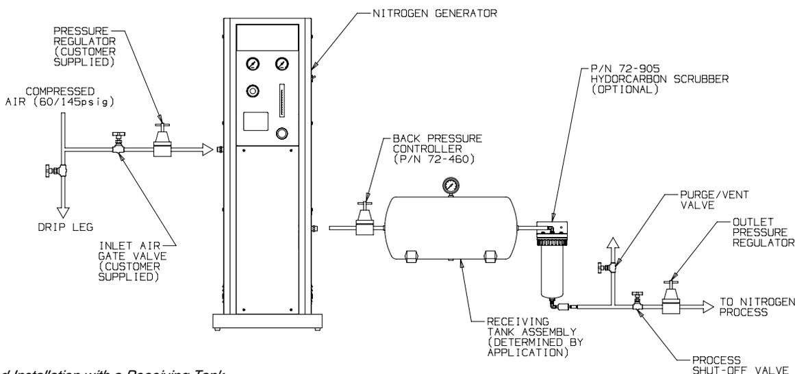
Figure 5 - Recommended Installation with a Receiving Tank
