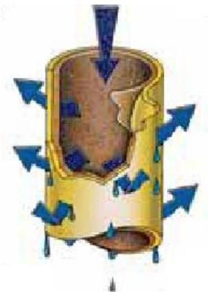
**Coalescing Filter** – Used to remove oil and water droplets, particulate matter from compressed air. The liquids drip to the bottom of the filter housing and are automatically emptied by a drain assembly.
